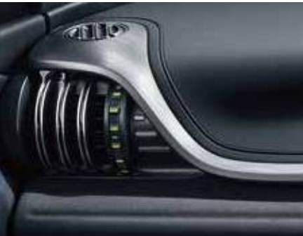
Dumbbell-style Air Conditioning Vents
